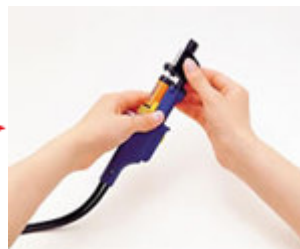
Firmly attach the nozzle remover to the nozzle cartridge as shown in the picture.
